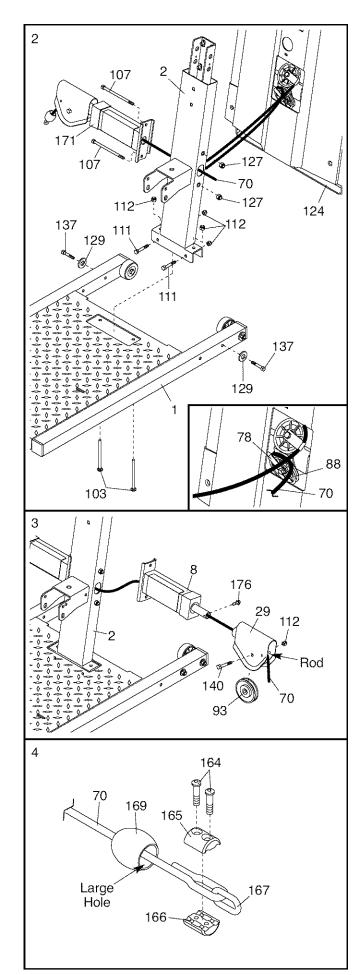
Remove the two M14 Nylon Locknuts (127).
